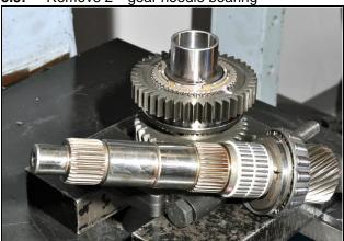
**5.11:** Press down on main shaft to remove 1st gear, 1-2 synchronizer, 1st gear bearing, 1-2 blocking rings, 2<sup>nd</sup> gear bearing journal, and thrust washer
