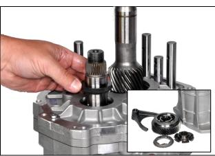
3.27: Remove 5th gear thrust washer
