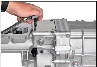
3.5: Remove four bolts to shift lug inspection cover
