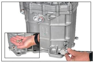
3.38: Remove two shift rail detent plugs
