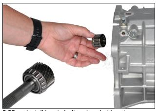
8.28: Install input shaft and pocket bearing
