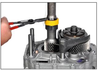
3.18: Remove speedometer gear snap ring
