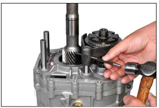
3.23: Remove 5th gear fork roll pin
