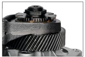
8.21: Install counter shaft locking nut
