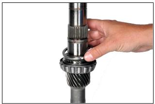
6.1: Install output shaft bearing
