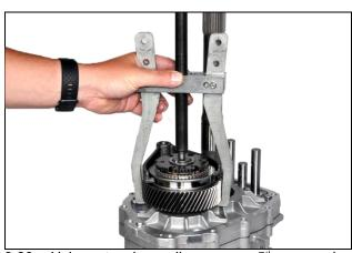
**3.26:** Using a two-jaw puller, remove 5<sup>th</sup> gear and synchronizer assembly
