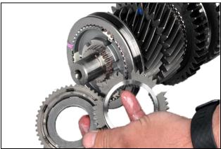
5.1: Remove 4<sup>th</sup> gear clutching teeth ring
