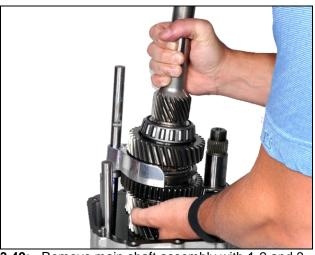
**3.40:** Remove main shaft assembly with 1-2 and 3-4 shift fork and rail assembly
