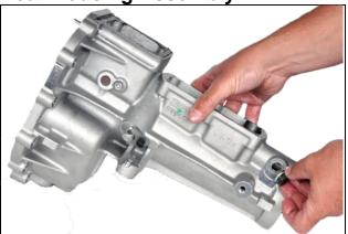
7.1: Install pipe plug. Torque to 15-25 lb-ft.
