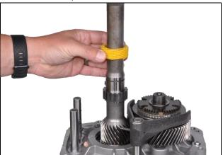
3.19: Remove mechanical speedometer gear
