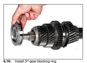
6.16: Install 3<sup>rd</sup> gear blocking ring
