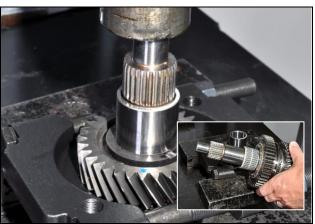
Install press plate under 2<sup>nd</sup> gear 5.7:
