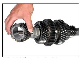
**6.15:** Install 3<sup>rd</sup> gear onto main shaft
