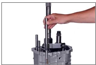
**8.4:** Install 5<sup>th</sup> and reverse gear fork and rail into main case
