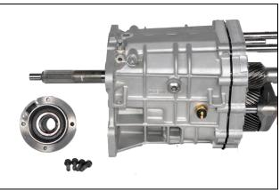
3.13: Remove front bearing retainer
