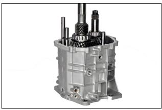
8.3: Install main shaft and fork assembly into main case. Use a 2 ½" (round) x 1" (thick) spacer on the table to hold main shaft.
