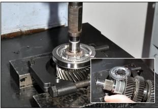
**5.4:** Install press plate under 3<sup>rd</sup> gear
