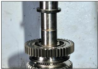
6.9: Install 2<sup>nd</sup> gear inner and outer blocking rings onto 1-2 synchronizer
