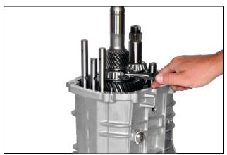
8.7: Install pivot pin snap ring
