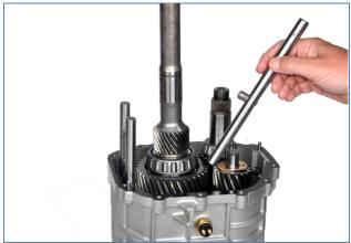
**3.34:** Rotate 5<sup>th</sup> reverse shift rail counter clockwise and remove from case
