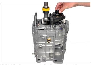
**3.16:** Position transmission in vertical position to access rear
