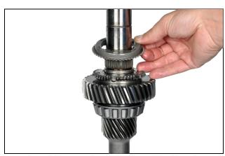
**6.6:** Install inner and outer 1st gear blocking ring
